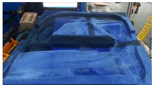
Figure 4. Dedicated Jig for Door-Trim Assembly
