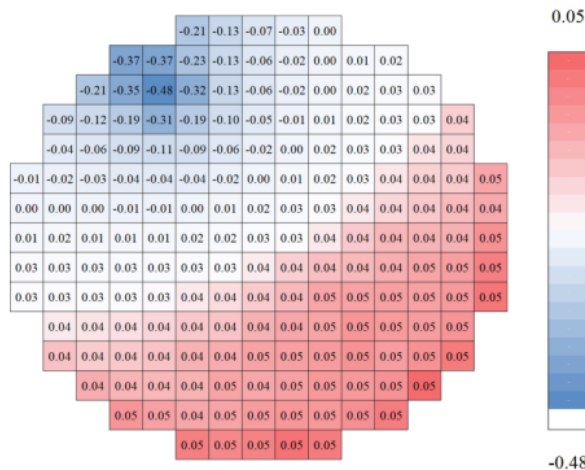
(c) Difference(b)-(a) Figure 4. Change of Assembly Power Distribution by Insertion of Rod Bank
