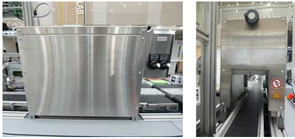
(a) Heat tunnel
