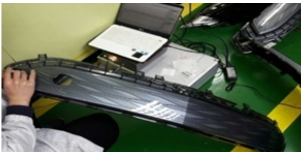
Figure 5. Penetration Film Thickness Measurement Using a Measuring Device
