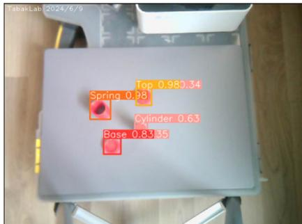
Figure 11. The Result of the Part Detection ML Prediction
