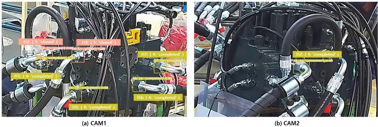
Figure 9. Results of the Automated Inspection by CAM1 and CAM2
