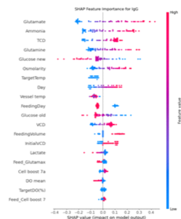
(c) Variable impact analysis for IgG prediction using a DNN model trained on integrated process variable and output feature data
