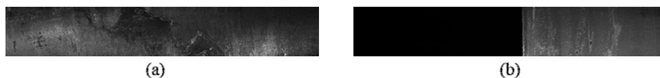
Figure 3. Sample images of Severstal Dataset. (a) a sample image filled with steel sheet surface only. (b) a sample image filled with steel sheet surface and invalid background (area of black color)
